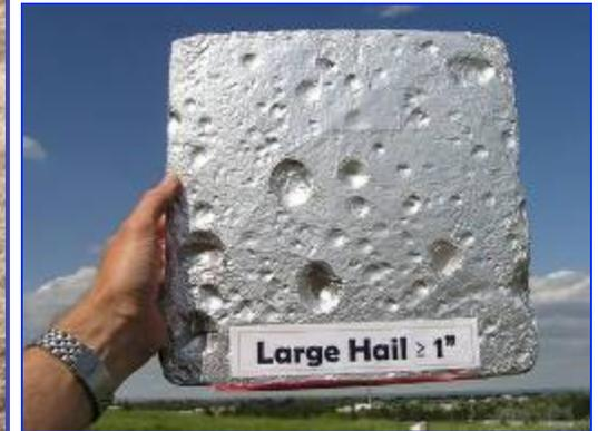
Aluminum foil-wrapped Styrofoam hail pads
