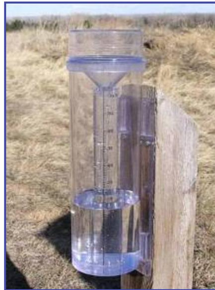
4-inch diameter high capacity rain gauges
