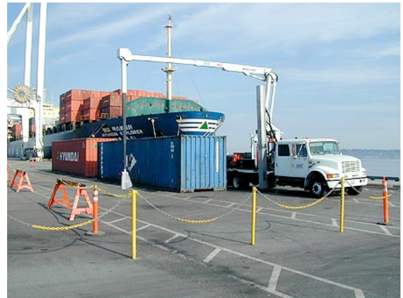
Mobile VACIS: truck-mounted gamma ray imaging system
