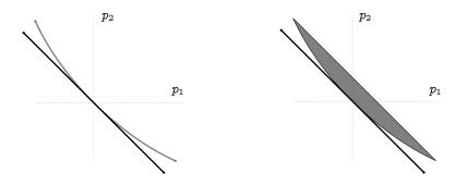
black: lossless, capacitated line; gray: AC power loss
