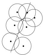
(A cylinder c of radius r contains a point q iff the axis of c stabs the ball of radius r centered at q)
