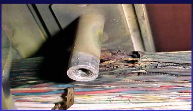
An arcing event has occurred. It is assumed that the arcing event began with one or two wire chaffing against the standoff. However, as a result of the arcing many wires in the bundle have failed. The possible effect of the failure depend on which systems are routed in the bundle.
