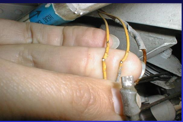
Insulation has faults. An EWIS failure probably has not occurred yet but the probability of an EWIS event is much higher. A common cause fault is indicated as the breach in the insulation line up.
