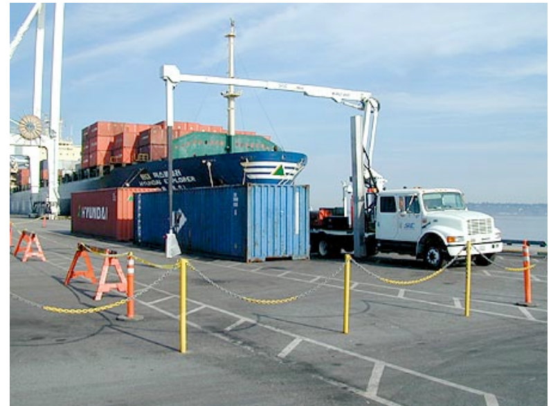
Mobile VACIS: truck-mounted gamma ray imaging system
