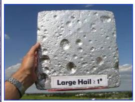
Aluminum foil-wrapped Styrofoam hail pads
